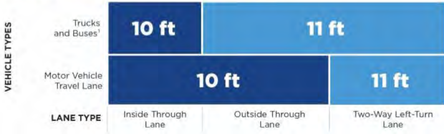
Figure 40: Recommended general-purpose lane widths
